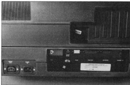
Rear view: the Advance ports, RGB, composite, TV, printer, joystick, cassette, RS232 and mains, are all clearly labelled.
